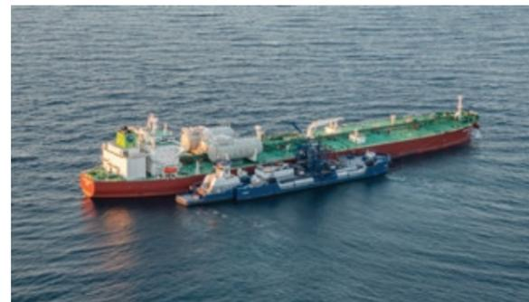
In October 2021, we completed our first ever LNG bunkering in the US, working in coordination with Shell to refuel the LNG dual-fuel Aframax tanker Pacific Ruby outside Port Canaveral in Florida. Six hundred metric tonnes of marine LNG was transferred onto the tanker from the Q-LNG 4000 bunker barge. The entire bunkering operations coordinated by AET and Shell and was safely and successfully completed in nine hours while Pacific Ruby was on its way from Houston bound for Rotterdam.
