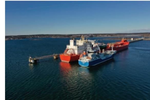
Eagle Balder completed her first two bunkering operations at the Port of Gothenburg, Sweden in early 2021. This LNG dual-fuel DPST is among the cleanest DPSTs ever built. The ship-to-ship bunkering operations were completed safely and simultaneously without interruption to the cargo operations. Prior to the operations, the crew and offshore personnel conducted careful and thorough risk assessment to ensure full compliance with the industry's best practices.
