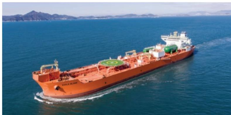
Through Dynamic Positioning technology, these vessels are able to maintain a fixed position without anchoring and load from offshore production facilities located in deepwater and/or harsh weather conditions.
